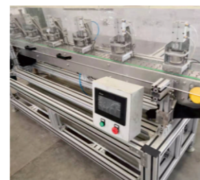
不锈钢平顶链磨损试验机 Abrasion Tester for Stainless Steel Flat Top Chain
